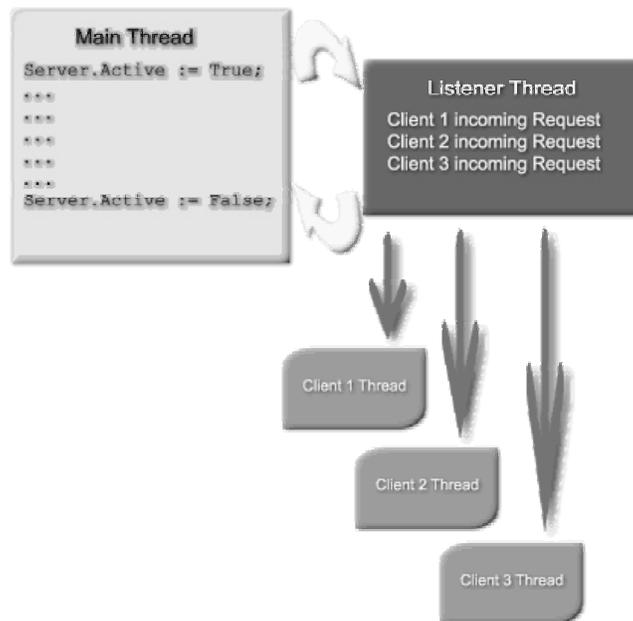
**Figure 20-1** Operation of `TIdTCPServer`
